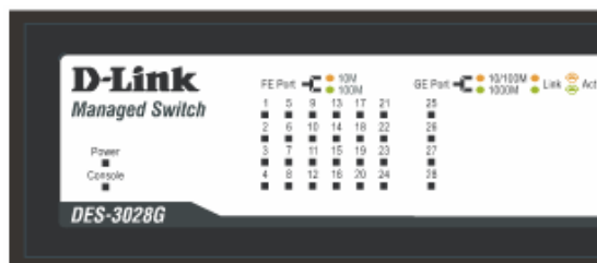
Figure 1- 3. LED Indicators on DES-3028G Switch
